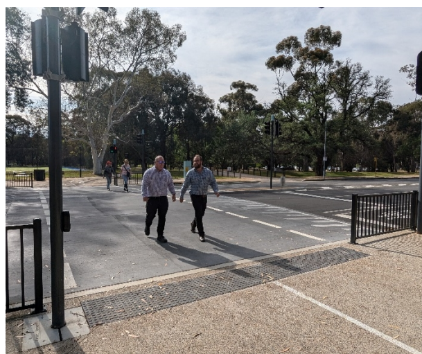
Bicycle Pedestrian Actuated Crossing (BPAC) with a raised safety platform on Hutt Road. This is an example of a primary Safe System aligned crossing outcome.
